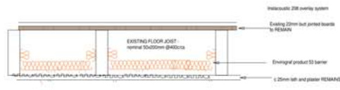
DETAIL 03 SUSPENDED TIMBER FLOOR PROPOSED UPGRADING USING ENVIROGRAF PRODUCT 53 - EXISTING LATH AND PLASTER CEILING RETAINED
